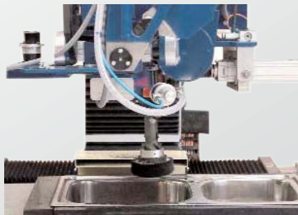
Bottom surface polishing. Bodenbearbeitung.
