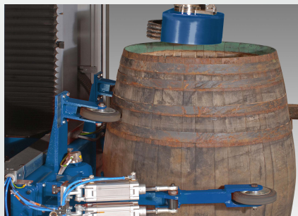
Flexible automatic clamping device for cask.
