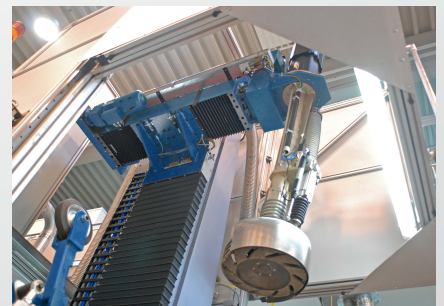
View of Z-Axis with Rasp tool.
