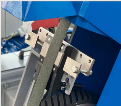
Schleifschuh Flat platen attachment
